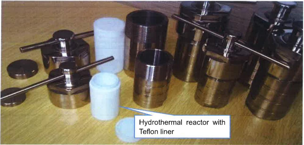
Hydrothermal reactor with Teflon liner
